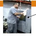
This bin has fold down door so the worker can get the product with less bending
