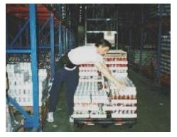
An adjustable height pallet jack with a turntable would allow this worker to turn and raise the load to get the product, instead of reaching.
